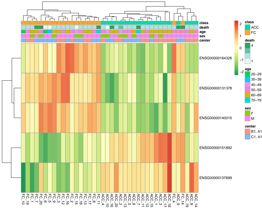
Figure 13: Clustergram. The clustergram is generated by using the expression values of the 5 predictors selected by DaMiR.FBest function. As for the heatmap generated by DaMiR.Allplot, 'class' and covariates are drawn as horizontal and color coded bars.
